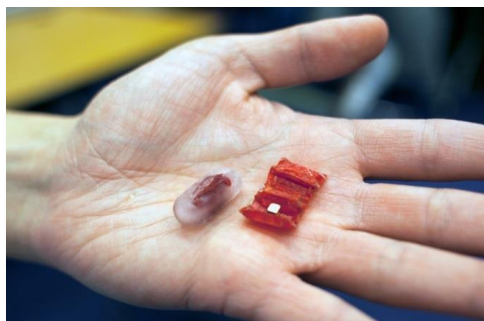
NSF-funded researchers have developed an origami robot that folds into an ingestible capsule. Credit: Melanie Gonick, MIT.
